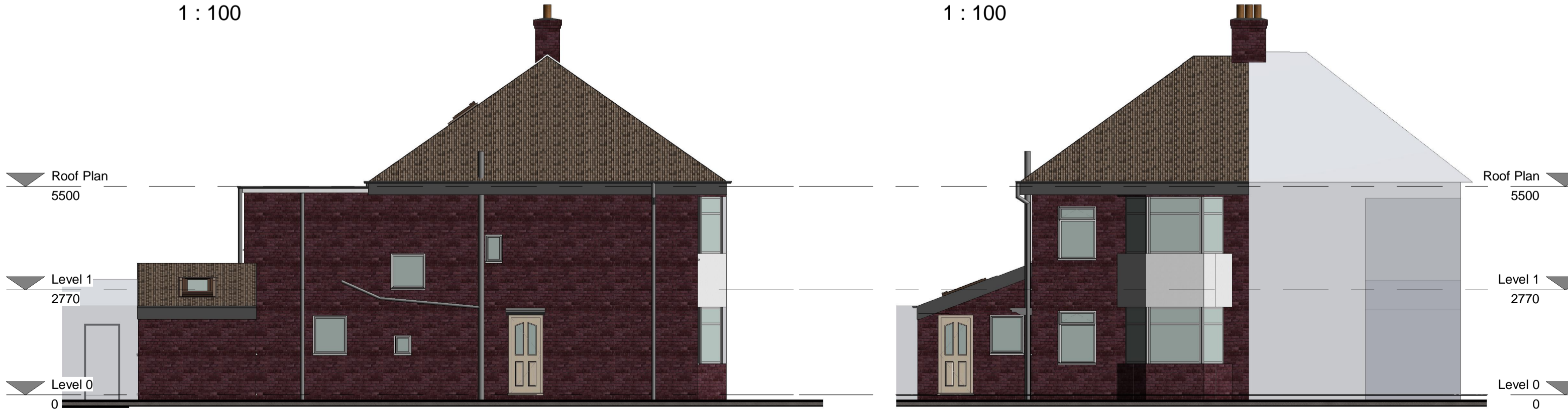
South West Elevation 1 : 100
